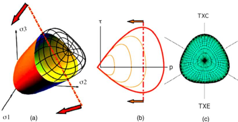
Fig. 1. (a) Yield surface with a high-pressure cap shown as a wireframe. (b) Meridional side view, with the hydrostat as abscissa. (c) Noncircular octahedral profile allowing for well-known extension-compression differences in brittle strength.
