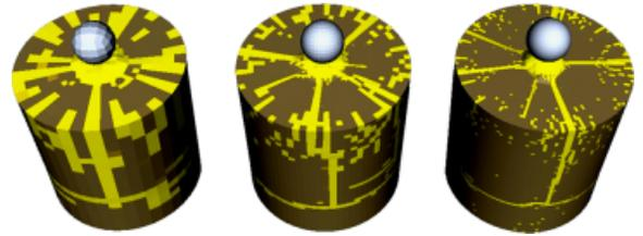
Fig. 6. Mitigating mesh dependency in three different resolution silicon carbide indentation simulations. Larger to smaller mesh sizes shown from left to right.
