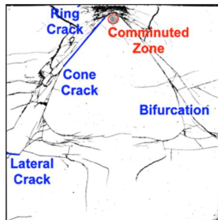
Fig. 7. Crosssectioned silicon carbide specimen with highlighted features.
