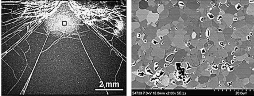
Fig. 8. Silicon carbide cross section of 500 m/s impact (left) and zoom in of comminuted zone (right).
