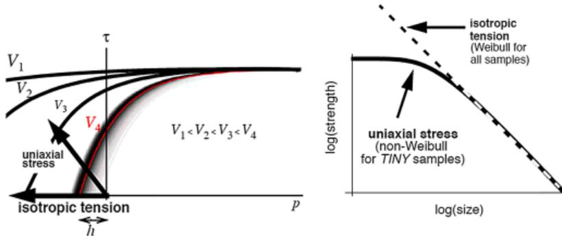
Fig. 2. The Weibull scale effect is applied only on the pressure intercept. The curved lines on the left plot are median limit surfaces for different specimen volumes showing that, as shown in the plot on the right, strength remains bounded for any stress path, such as uniaxial stress, having a deviatoric component.
