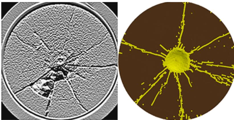
Fig. 9. X-ray computed tomography image of top surface cracking (left) and corresponding simulation (right) from a 385 m/s impact of silicon carbide.
