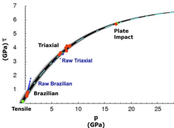
Fig. 3. Meridional view of the Kayenta material model and experiments for silicon carbide.
