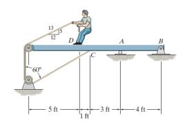
Equations of Equilibrium and Friction: When the boy is on the verge to slipping, then  $F_D=(\mu_s)_D N_D=0.4N_D$ . From FBD (a),
