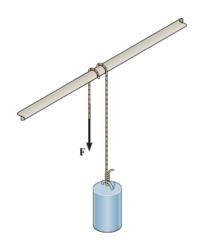
Frictional Force on Flat Belt: Here,  $T_1 = F$  and  $T_2 = 250(9.81) = 2452.5$  N. Applying Eq. 8-6, we have
