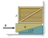
Free - Body Diagram. Since the crate is on the verge of sliding up and the wedge is on the verge of sliding to the right, the frictional force  $\mathbf{F}_A$  on the crate must act downward and forces  $\mathbf{F}_B$  and  $\mathbf{F}_C$  on the wedge must act to the left as indicated on the free - body diagrams as shown in Figs. a and b. Also,  $F_A = \mu_s N_A = 0.3 N_A$ ,  $F_B = \mu_s N_B = 0.3 N_B$ , and  $F_C = \mu_s N_C = 0.3 N_C$ .
