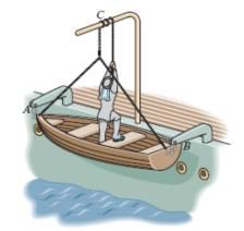
Frictional Force on Flat Belt: If the normal force between the man and the boat is equal to zero, then,  $T_1=130$  lb and  $T_2=500$  lb. Applying Eq. 8-6, we have
