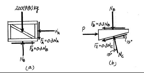
\*8–72. If the horizontal force P is removed, determine the largest angle  $\theta$  that will cause the wedge to be self-locking regardless of the magnitude of force F applied to the handle. The coefficient of static friction at all contacting surfaces is  $\mu_s = 0.3$ .
