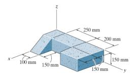
Centroid: Since the block is made of a homogeneous material, the center of mass of the block coincides with the centroid of its volume. The centroid of each composite segment is shown in Fig. a.
