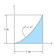
Differential Element: The area element parallel to the y axis shown shaded in Fig. a will be considered. The area of the element is
