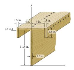
Centroid: The centroid of each composite segment is shown in Fig. a.
