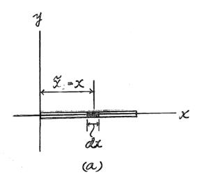
9–7. Locate the centroid  $\overline{x}$  of the circular rod. Express the answer in terms of the radius r and semiarc angle  $\alpha$ .
