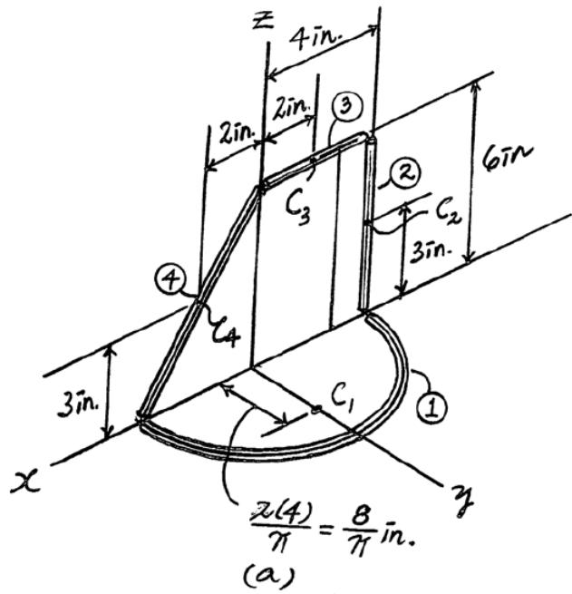
\*9-56. Locate the centroid  $\bar{y}$  of the cross-sectional area of the built-up beam.
