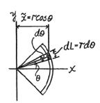
•9–9. Determine the area and the centroid  $(\overline{x}, \overline{y})$  of the area.
