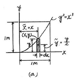
\*9–24. Locate the centroid  $(\overline{x}, \overline{y})$  of the area.
