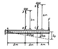
**2–7.** The two wires are connected together at A. If the force  $\mathbf{P}$  causes point A to be displaced horizontally 2 mm, determine the normal strain developed in each wire.
