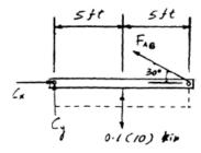
\*3-24. The beam is supported by a pin at C and an A-36 steel guy wire AB. If the wire has a diameter of 0.2 in., determine the distributed load w if the end B is displaced 0.75 in. downward.
