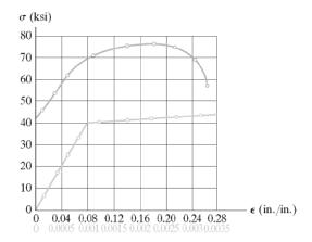
Modulus of Elasticity : From the stress – strain diagram,  $\sigma$  = 40 ksi when  $\varepsilon$  = 0.001 in./in.
