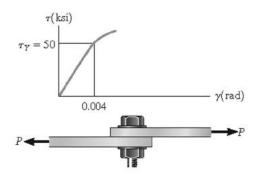
Modulus of Rigidity: From the stress - strain diagram,
