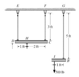
Internal Forces in the wires :
