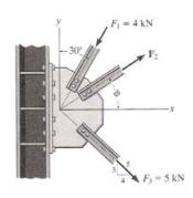
**Rectangular Components:** By referring to Fig. a, the x and y components of  $F_1$ ,  $F_2$ ,  $F_3$ , and  $F_R$  can be written as
