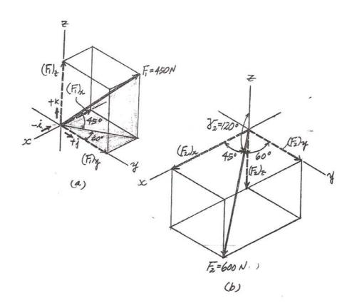
\*2-60. Determine the magnitude and coordinate direction angles of the resultant force acting on the bracket.
