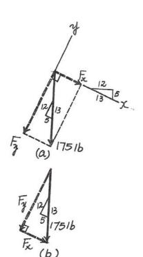
**2–38.** If  $\phi=30^\circ$  and the resultant force acting on the gusset plate is directed along the positive x axis, determine the magnitudes of  $\mathbf{F}_2$  and the resultant force.
