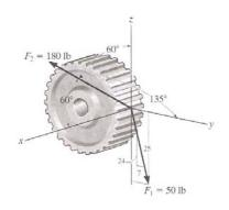
\*2–68. The spur gear is subjected to the two forces caused by contact with other gears. Determine the resultant of the two forces and express the result as a Cartesian vector.
