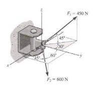
Rectangular Components: Since  $\cos^2\alpha_2 + \cos^2\beta_2 + \cos^2\gamma_2 = 1$ , then  $\cos\gamma_{2z} = \pm\sqrt{1-\cos^245^\circ - \cos^260^\circ} = \pm0.5$ . However, it is required that  $\gamma_2 > 90^\circ$ , thus,  $\gamma_2 = \cos^{-1}(-0.5) = 120^\circ$ . By resolving  $F_1$  and  $F_2$  into their x, y, and z components, as shown in Figs. a and b, respectively  $F_1$  and  $F_2$  can be expressed in Cartesian vector form as
