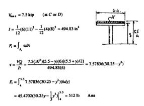
\*7-36. The beam is constructed from two boards fastened together at the top and bottom with two rows of nails spaced every 6 in. If each nail can support a 500-lb shear force, determine the maximum shear force V that can be applied to the beam.
