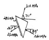
9-22. The clamp bears down on the smooth surface at E by tightening the bolt. If the tensile force in the bolt is 40 kN, determine the principal stresses at points A and B and show the results on elements located at each of these points. The cross-sectional area at A and B is shown in the adjacent figure.
