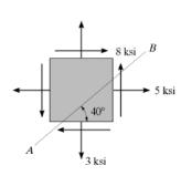
$\frac{\sigma_x + \sigma_y}{2} = \frac{5+3}{2} = 4 \text{ ksi}$   $R = \sqrt{(5-4)^2 + 8^2} = 8.0623$   $\phi = \tan^{-1} \frac{8}{(5-4)} = 82.875^\circ$   $2\theta = 2(130^\circ) = 260^\circ$
