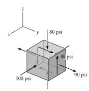
Construction of the Circle: Mohr's circle for the element in the y - z plane is drawn first. In accordance with the sign convention,  $\sigma_y = 90$  psi,  $\sigma_z = -80$  psi, and  $\tau_{yz} = 40$  psi. Hence,
