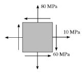
Construction of the Circle: In accordance with the sign convention,  $\sigma_x = 10$  MPa,  $\sigma_y = 80$  MPa and  $\tau_{xy} = -60$  MPa. Hence,
