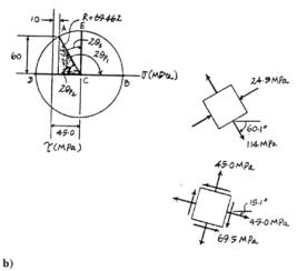
Maximum In - Plane Shear Stress: Represented by the coordinate of point E on the circle.
