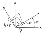
\*10-8. The state of strain at the point on the gear tooth has the components  $\epsilon_x = 520(10^{-6}), \ \epsilon_y = -760(10^{-6}),$  $\gamma_{xy} = -750(10^{-6})$ . Use the strain-transformation equations to determine (a) the in-plane principal strains and (b) the maximum in-plane shear strain and average normal strain. In each case specify the orientation of the element and show how the strains deform the element within the x-y plane.
