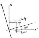
**10–23.** The strain at point A on the bracket has components  $\epsilon_x = 300(10^{-6})$ ,  $\epsilon_y = 550(10^{-6})$ ,  $\gamma_{xy} = -650(10^{-6})$ ,  $\epsilon_z = 0$ . Determine (a) the principal strains at A, (b) the maximum shear strain in the x-y plane, and (c) the absolute maximum
