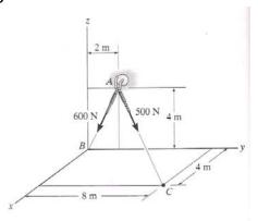
$$r_{AB} = (-2j-4 \text{ k})\text{m}; \quad r_{AB} = 4.472 \text{ m}$$
