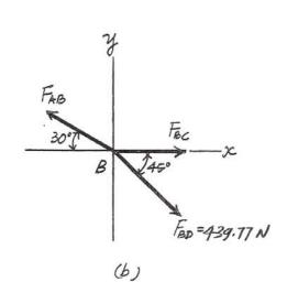
3-46. Determine the maximum mass of the crate so that the tension developed in any cable does not exceeded 3 kN.
