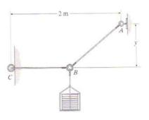
Equations of Equilibrium: Applying the equations of equilibrium along the x and y axes to the free - body diagram in Fig. (a),
