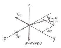
\*3–52. Determine the force in each of the three cables needed to lift the tractor which has a mass of 8 Mg.
