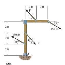
b) By resolving the 150-1b and 200-1b couples into their x and y components, Fig. a, and summing the moments of these force components algebraically about point A,
