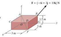
**4–54.** Determine the magnitude of the moments of the force  $\mathbf{F}$  about the x, y, and z axes. Solve the problem (a) using a Cartesian vector approach and (b) using a scalar approach.
