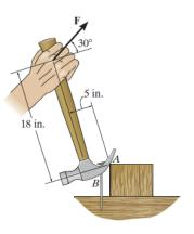
Resolving the 20 - 1b force into components parallel and perpendicular to the hammer, Fig. a, and applying the principle of moments,
