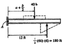
\*4-156. Replace the loading by an equivalent resultant force and couple moment acting at point B.
