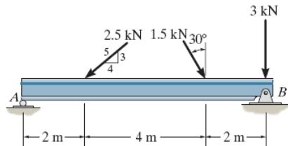
$$\rightarrow \sum F_x = \Sigma F_x; \quad F_{R_x} = 1.5 \sin 30^\circ - 2.5 \left(\frac{4}{5}\right) \\ = -1.25 \text{ kN} = 1.25 \text{ kN} \leftarrow$$
