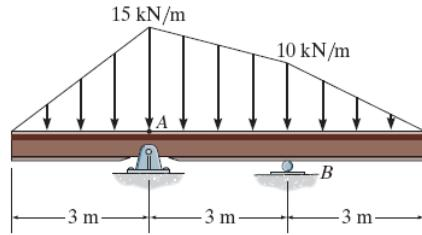
**Loading:** The distributed loading can be divided into four parts as shown in Fig. *a*. The magnitude and location of the resultant force of each part acting on the beam are also indicated in Fig. *a*.
