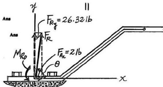
**4-110.** Replace the force and couple moment system acting on the overhang beam by a resultant force and couple moment at point A.
