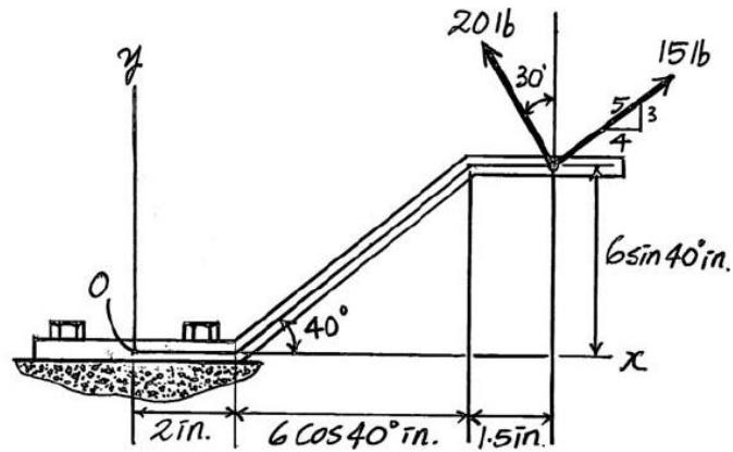
$$\rightarrow F_{Rx} = \Sigma F_x; \quad F_{Rx} = \frac{4}{5}(15) - 20 \sin 30^\circ = 2 \text{ lb}$$
