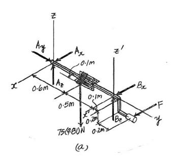
\*5–72. Determine the components of reaction acting at the smooth journal bearings A, B, and C.
