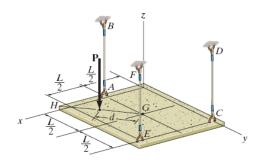
**Equations of Equilibrium:** From the free - body diagram, Fig. a,  $T_{AB}$  can be obtained by writing the moment equation of equilibrium about the x' axis.
