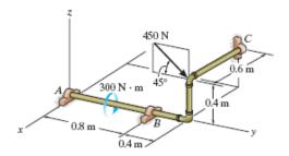
**Equations of Equilibrium:** From the free - body diagram of the shaft, Fig. a,  $C_y$  and  $C_z$  can be obtained by writing the force equation of equilibrium along the y axis and the moment equation of equilibrium about the yaxis.
