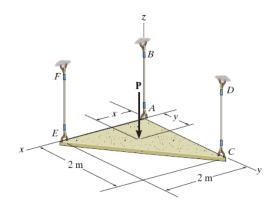
**Equations of Equilibrium:** From the free - body diagram of the plate, Fig. a, and writing the moment equations of equilibrium about the x' and y' axes,
