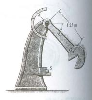
18-15. The hand winch is used to lift the 50-kg load. Determine the work required to rotate the handle five revolutions. The gear at A has a radius of 20 mm.
