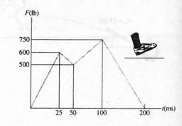
\*15-8. During operation the breaker hammer develops on the concrete surface a force which is indicated in the graph. To achieve this the 2-lb spike S is fired from rest into the surface at 200 ft/s. Determine the speed of the spike just after rebounding.
