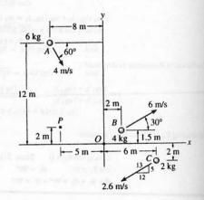
\*15-96. Determine the total angular momentum  $\mathbf{H}_O$  for the system of three particles about point O. All the particles are moving in the x-y plane.
