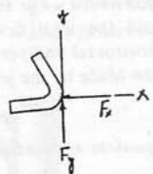
**15-113.** Water is flowing from the 150-mm-diameter fire hydrant with a velocity  $v_B = 15 \text{ m/s}$ . Determine the horizontal and vertical components of force and the moment developed at the base joint  $A$ , if the static (gauge) pressure at  $A$  is  $50 \text{ kPa}$ . The diameter of the fire hydrant at  $A$  is  $200 \text{ mm}$ .  $\rho_w = 1 \text{ Mg/m}^3$ .
