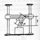
\*16-36. The block moves to the left with a constant velocity  $\mathbf{v}_0$ . Determine the angular velocity and angular acceleration of the bar as a function of  $\theta$ .
