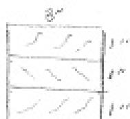
A "lam" beam is made up of three 1 in. x 3 in. (full size) pieces of wood bonded together to form the beam cross-section shown. If the beam is used in an application where  $M_{max} = 22,000$  in-lbs and  $V_{max} = 4000$  lbs. Determine (a) the maximum tensile stress, (b) the maximum compressive stress and (c) the shear stress in the adhesive used to bond the pieces of wood.
