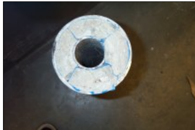
Step 6: After concrete has cured – cut off ends: done
