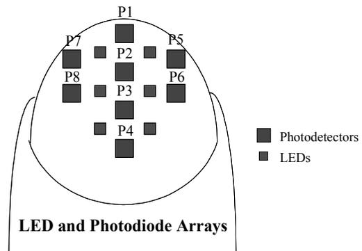
Figure 15. Sensor arrangement.
