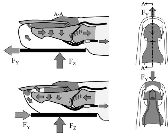
Figure 14. Longitudinal shear mechanism.
