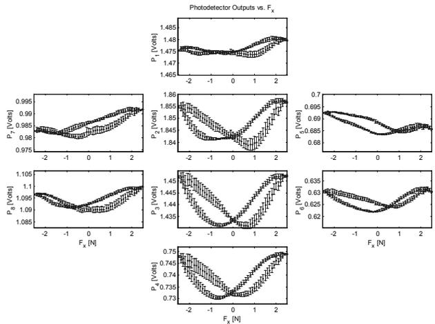
Figure 18. Sensor response to lateral shear.
