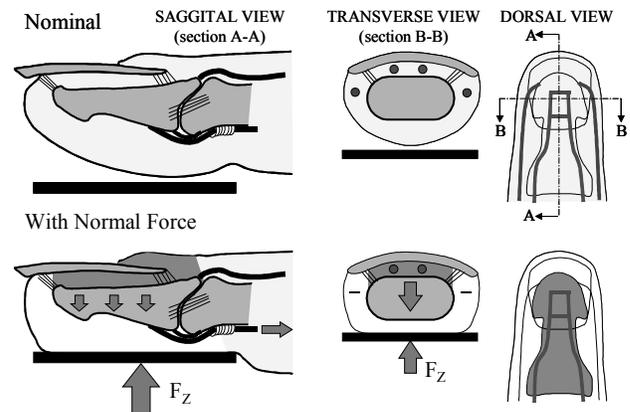
**Figure 11. Normal touch mechanism.**
